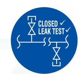
Always check that equipment is pressure-free and provide safe isolation before starting maintenance work.
